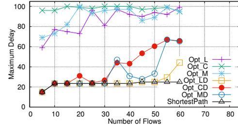
Fig. 9. Maximum delay of flows for different objective functions
