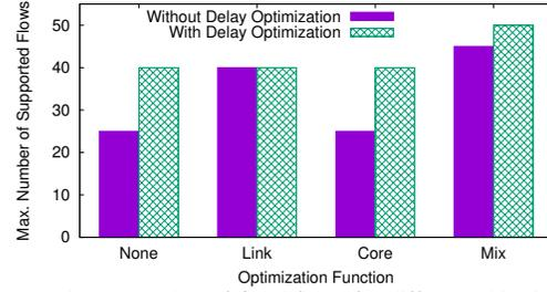
Fig. 3. Maximum number of fitted flows for different objective functions
