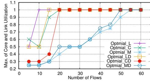
Fig. 8. Max. core and link utilization for different objective functions
