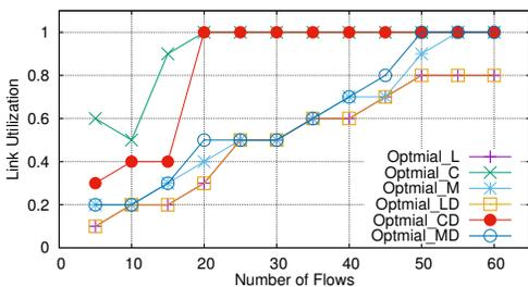
Fig. 7. Max. link utilization for problems with different objective functions
