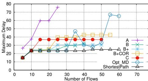
Fig. 12. Maximum flows' delay for different algorithms
